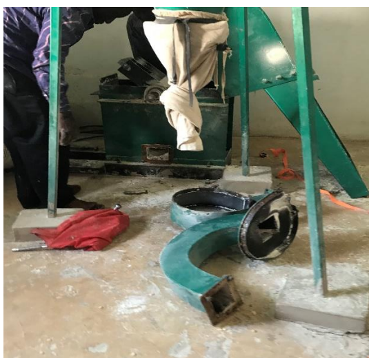
Figure 2. Assembling of hammer mill flour
