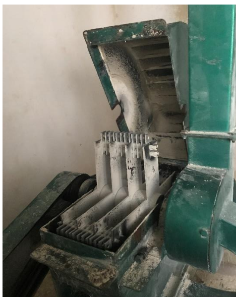
Figure 1: Diagrammatic representation of hammer mill
