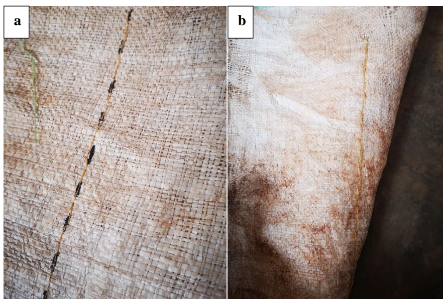
Figure 3. Picture (a) shows the sewing line in yellow on one side of the sisal bag. Picture (b) shows the sewing line in yellow on the opposite side.
