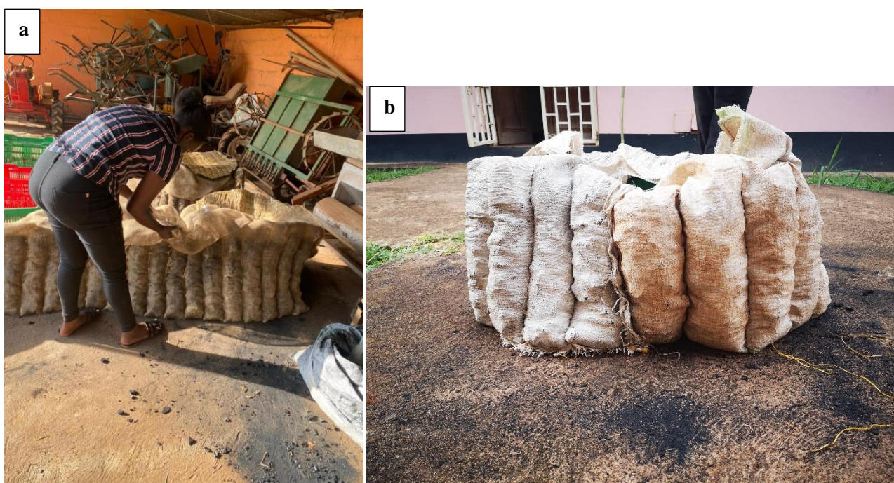
Figure 4. Picture (a) shows the process of filling the burlap blanket by hand. Picture (b) shows the finished charcoal cooling blanket made with sisal bags.
