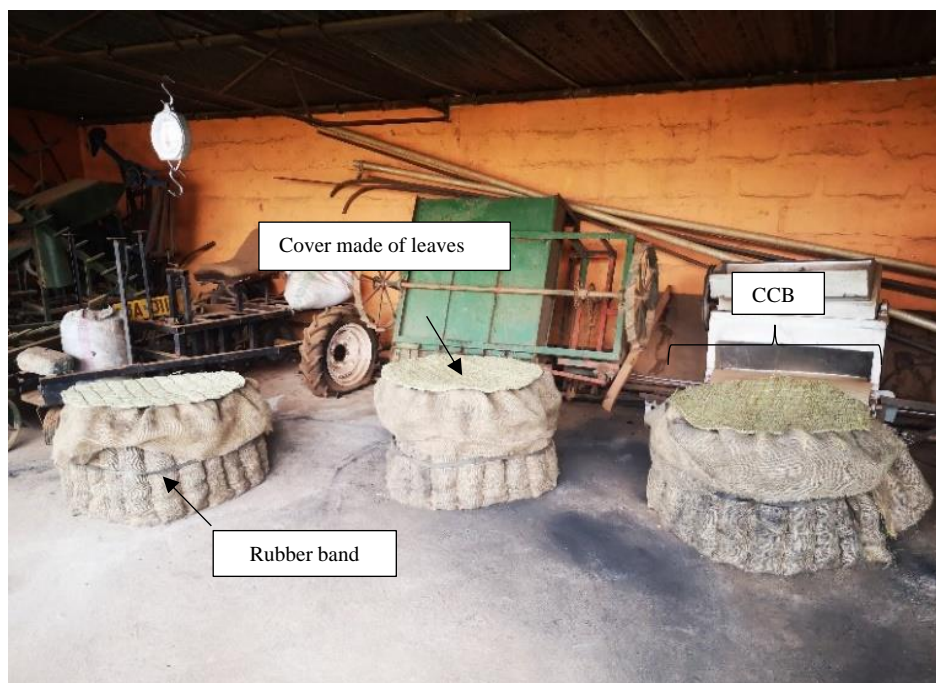
Figure 6. Three finished blankets tested at Makerere University. It is visible the rubber strap tied around and the leaf cover on top.
