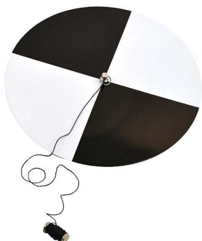
Fig. 8: Secchi Disk for measuring pond water turbidity
