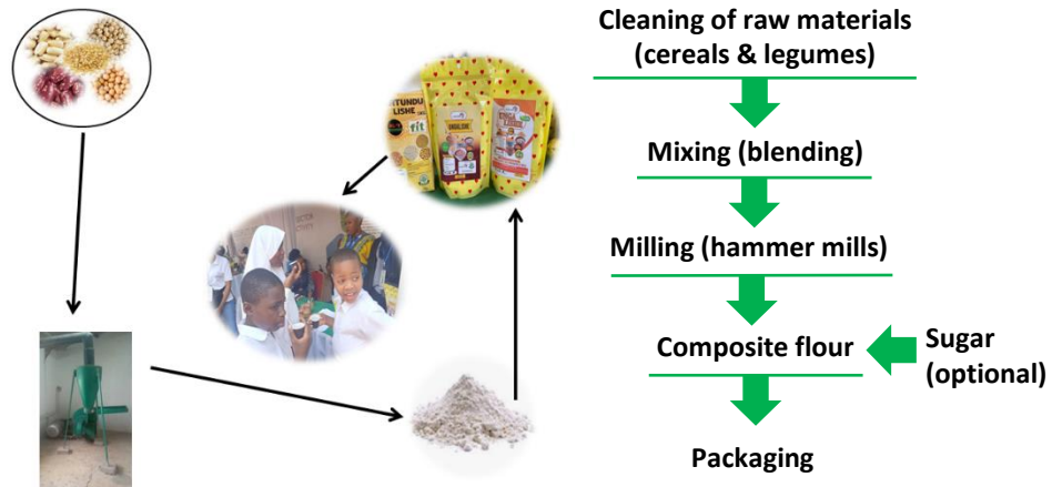
Figure 1. Composite flour production scheme (left) and flow diagram (right)
