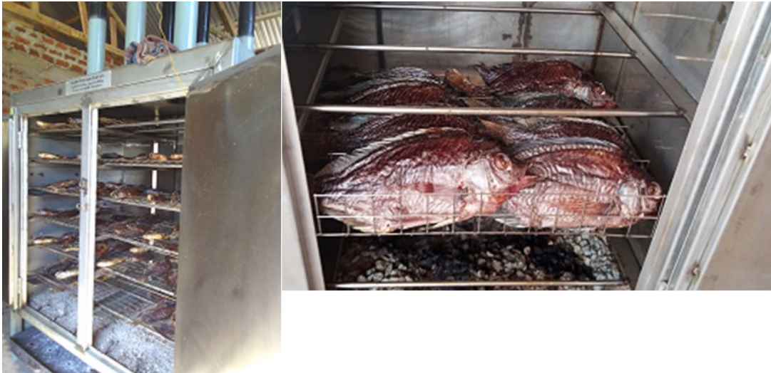
Fig 3. Smoking of fish using NARO PAH-Safe Fish Smoking Kiln
