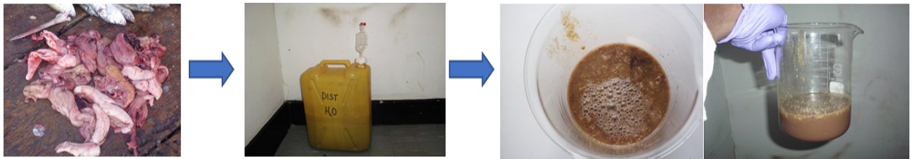
Fig. 4 Preparation of fish hydrolysate by Anaerobic Fermentation of Fish Guts using LAB
