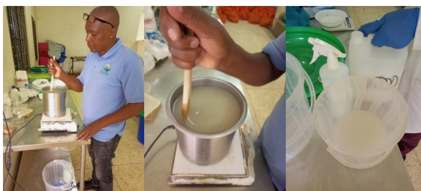
Figure 8. Preparation of cassava starch/chitosan-based coating.
